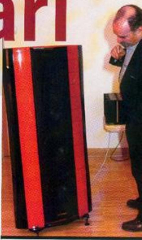
early attempt at making a large speaker shallow enough to wall- or shelf-mount, while retaining enough enclosure volume to allow it to load a massive woofer.
